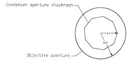
Note 1—The values shown for the radius of the condenser aperture diaphragm and the radius of the objective aperture are dimensionless. These values are given only to show the two-third ratio of the radii.
