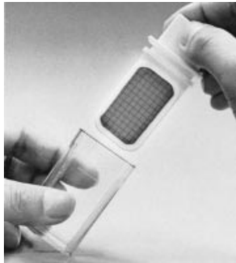
(d) Insert the sampler into the empty case and then place in the incubator.
