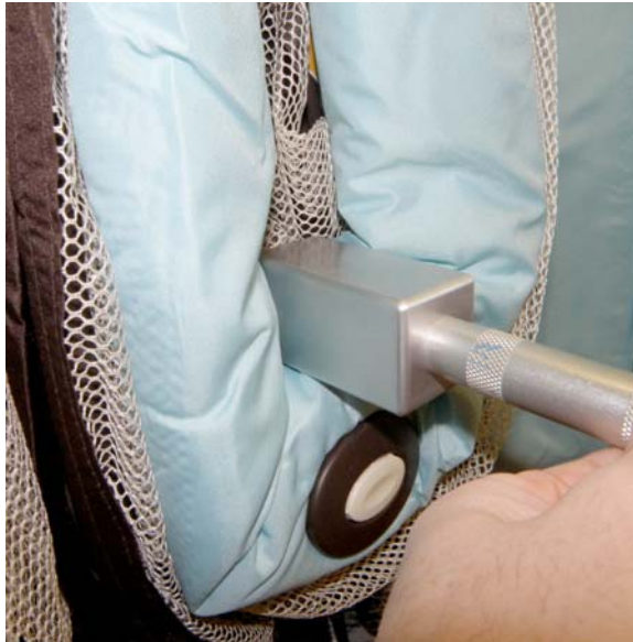
FIG. A1.37 Horizontal Spacing Probe Inserted Between Top Rail Segments per 8.29.1.4
