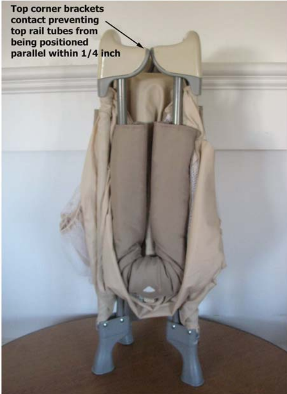
FIG. A1.36 Example of Folded Product whose Top Rails cannot be Made Parallel
