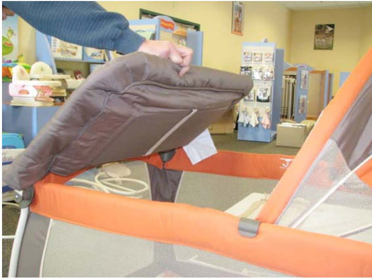
FIG. A1.7 Accessory That Attaches to the Play Yard on one Side and Rests on the Play Yard on the Other Side
