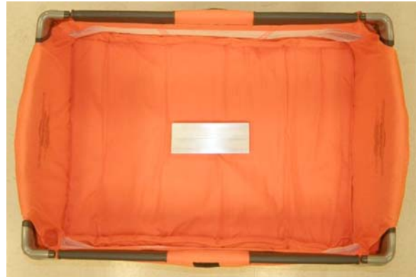
FIG. A1.42 Test Mass Positioned for Bassinet/Cradle Accessory Sleep Surface Test
