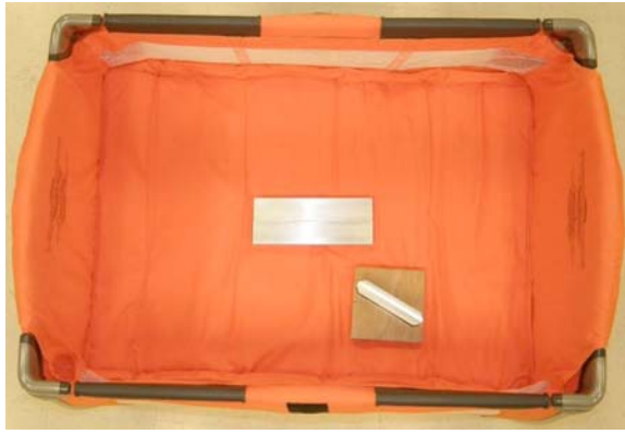
FIG. A1.43 Bassinet/Cradle Accessory Sleep Surface Test Angle Measurement
