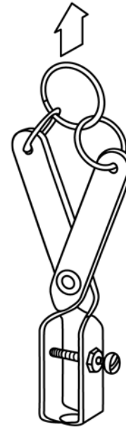
FIG. 8 Tension Test Adapter/Clamp
