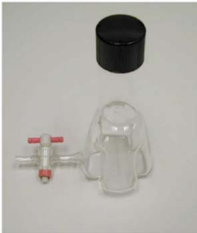
FIG. 1 The Baffled Flask Vessel with the Addition of a Stopcock and a Withdrawal Tube
