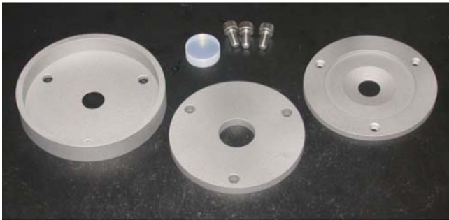
FIG. 11 Stainless Steel Clamping Top and Bottom along with Septum and Septum Restrictor
