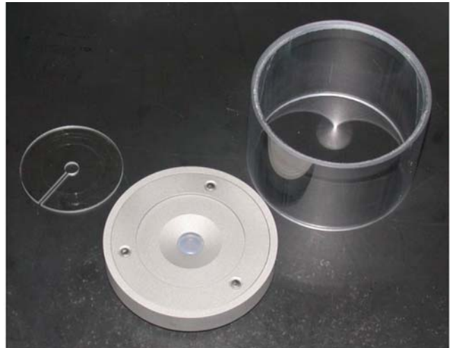
FIG. 12 Clamped Septum with Guide Template and Cylinder
