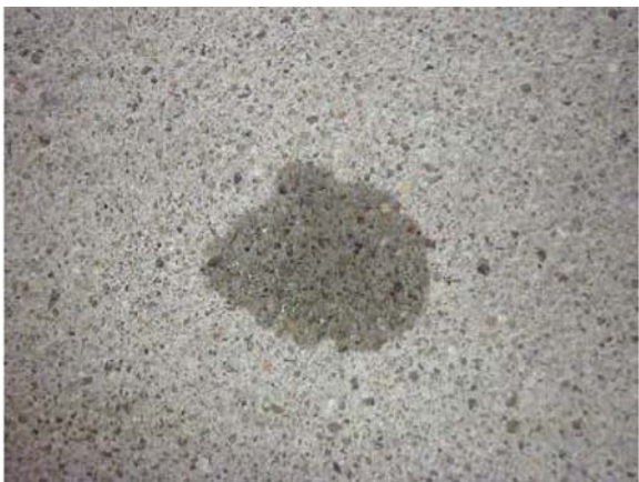
FIG. 3 Absorptive Concrete Surface
