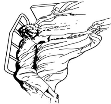
FIG. X1.3 Zone 3 – Entrapment Between the Product and Mattress
