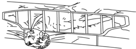
FIG. X1.2 Zone 2 – Entrapment Under the Product, Between the Supports or Next to a Single Support
