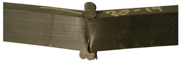
Figure X1.1B - Type II side bend result showing partial tear within the combined fusion bead zone
