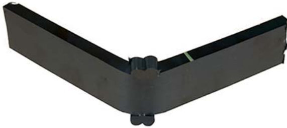
Figure X1.1A - Type I side bend result showing ductile deflection with no indication of tears, splits or breaks
