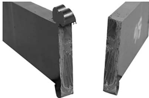
Figure X1.1C - Type III test result showing break within the combined fusion bead zone
