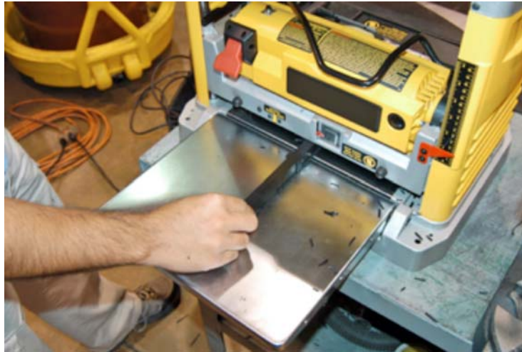
FIG. 7 Electric Planer for Side Bend Specimen Preparation
