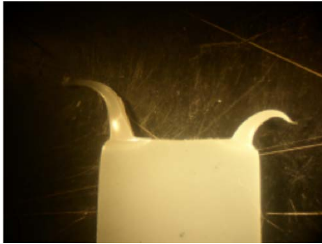
FIG. 5 "Double-horned" Failure Due to Crack Originating From a Contaminant
