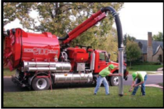
FIG. 3 Vacuum Excavation Equipment
