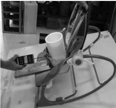
FIG. 11 Forward Stability Test for Infant/Toddler Rockers
