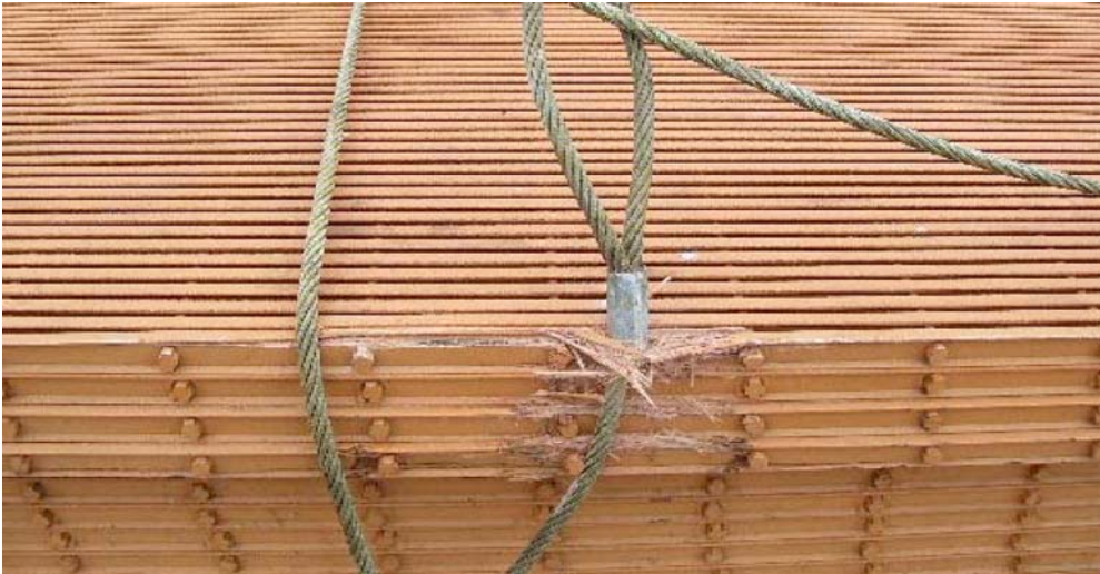
FIG. X1.13 Damage Caused by Incorrect Handling of FRP Gratings
