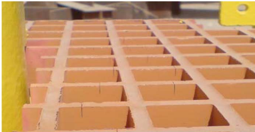
FIG. X2.4 Vertical Cracks in Molded Cells
