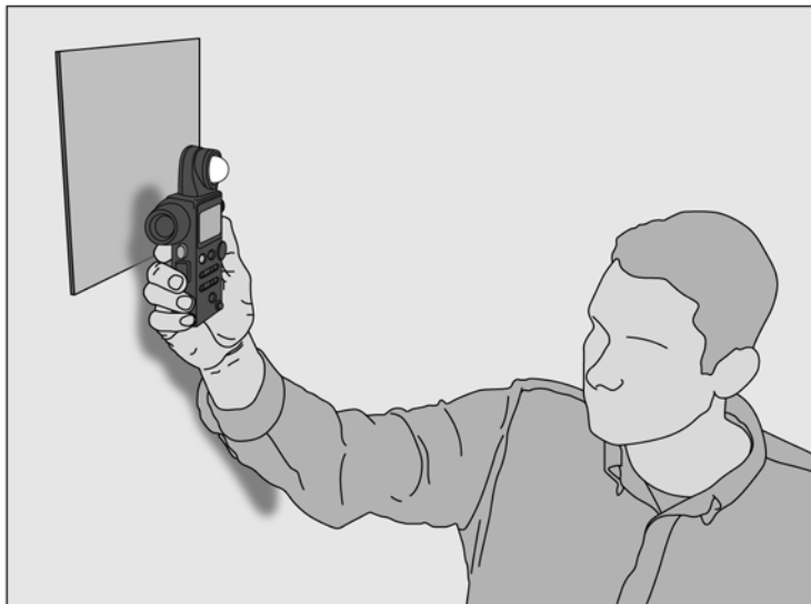
FIG. 13 Incident Light Meter Positioning
