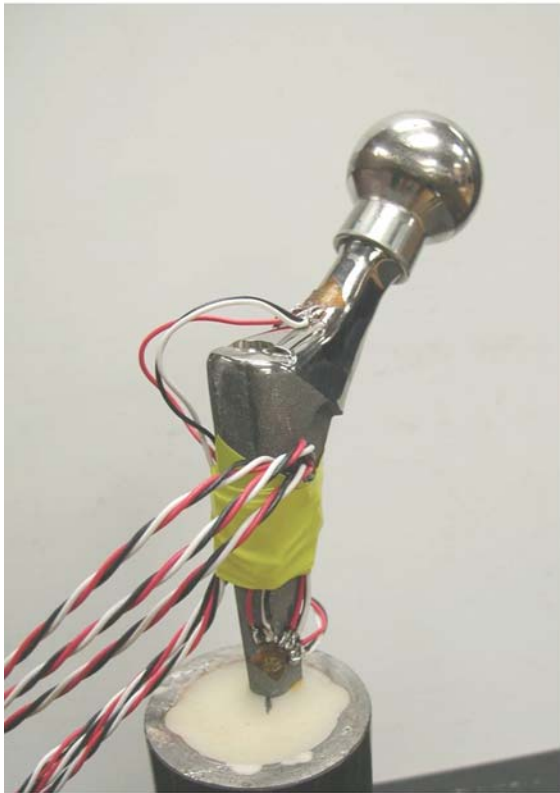
FIG. X4.1 Laboratory 1—Conventional Strain Gage (left) and FEA (right) Comparison for the Grit Blasted Ti-6Al-4V Hip Stem (Note 1)
