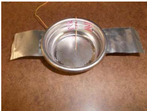
FIG. 3 Thermocouple Location in Portafilter for Monitoring Single Cup (Type I) Brewer Dispensing Temperature
