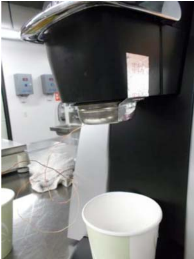
FIG. 2 Portafilter Installation on Single Cup (Type I) Brewer
