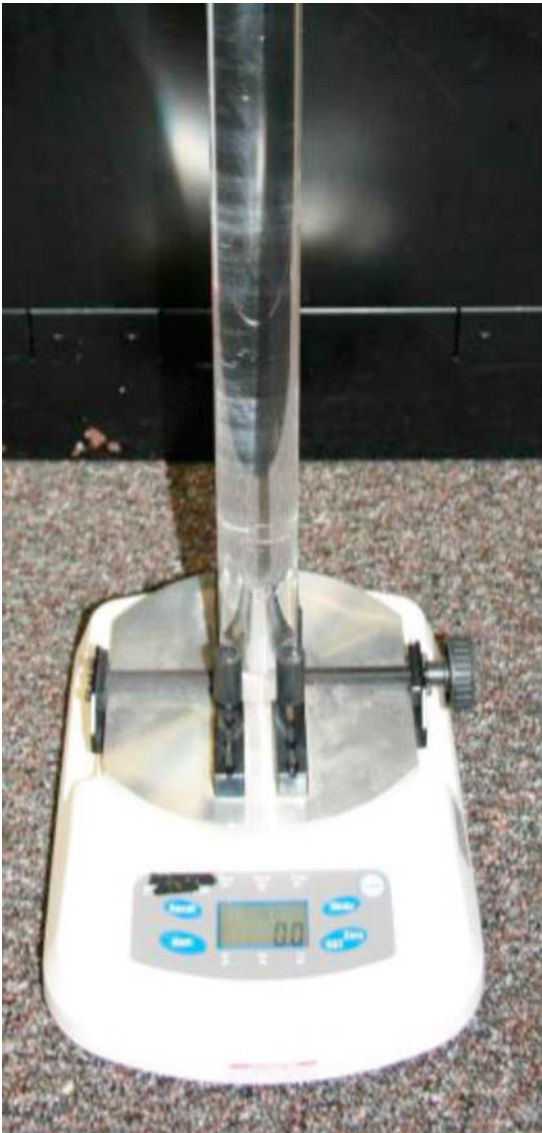
FIG. 1 Acrylic Rod Attached to a Torque Meter
