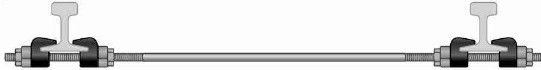
FIG. 1 Gauge Rods (installed on rails, ties and tie plates not shown)
