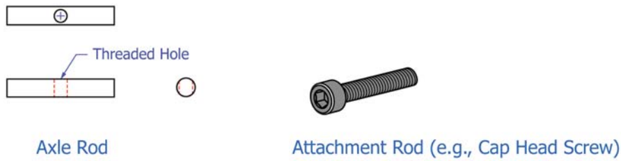
FIG. A2.2 Example Bending Axle Rod and Attachment Rod (quantity =4)
