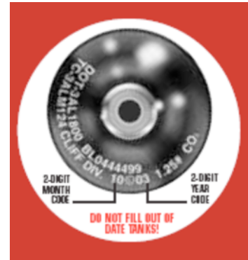
FIG. 6 Valve/Cylinder Rotation Indicator Marking
