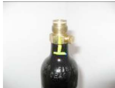
FIG. 6 Valve/Cylinder Rotation Indicator Marking
