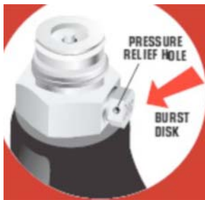
FIG. 2 Pin Valve Showing Example of Burst Disk Assembly Relief Hole
