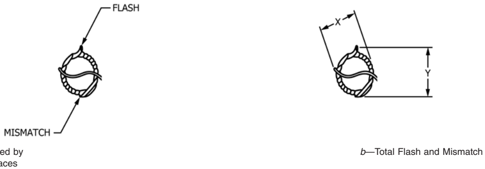
FIG. 2 Fitting Insert Dimensions and Tolerances
