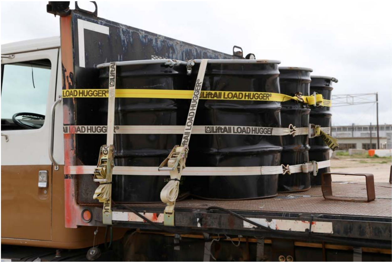
FIG. 2 Typical Ballast Attachment, Rear View
