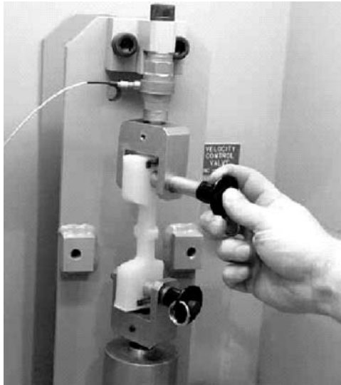
FIG. 5 Pin the Specimen in the Testing Machine
