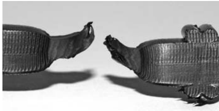
FIG. 2 Ductile Rupture Outside Fusion Interface
