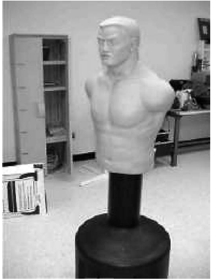
NOTE 1—This figure illustrates typical device that is acceptable. FIG. 5 Test Torso
