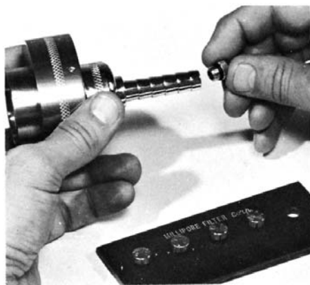
FIG. 6 Inserting a Typical Orifice
