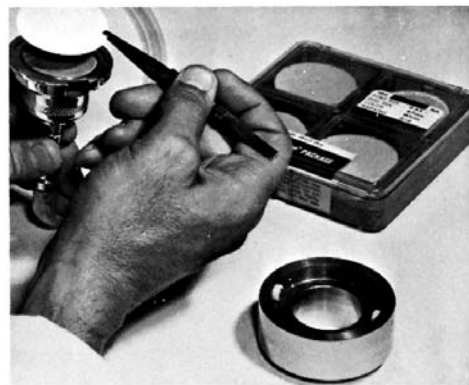
FIG. 7 Placing the Filter on a Typical Screen Support
