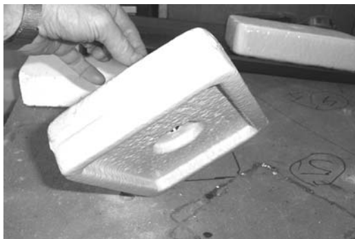
FIG. 1 Typical RH Hood Showing Air Chamber
