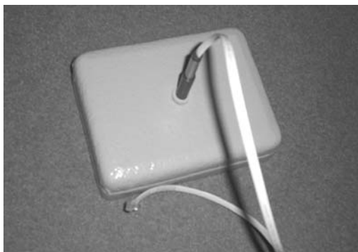
FIG. 2 Typical RH Hood Showing RH Probe Positioned in Hood
