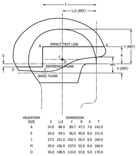
Note 1—The center of impact can be anywhere on or above the test line.
