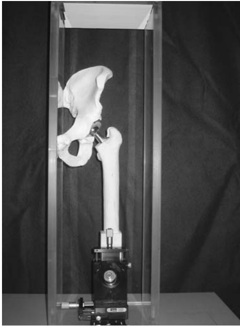
FIG. 1 Phantom Model Capable of Moving the Femoral Head by Small Discrete Three Dimensional Displacements
