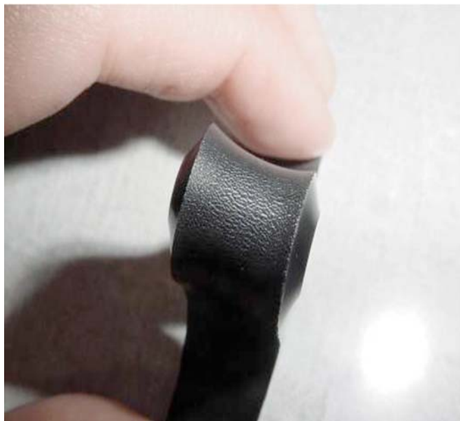
FIG. X3.1 Strained inner surface of pipe following bend-back showing microcracking of surface
