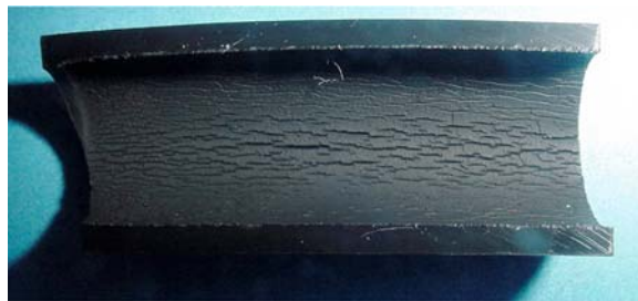
FIG. X3.4 Optical image of inner surface (Stage III)
