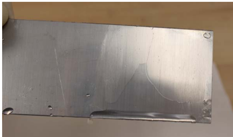
FIG. 3 Aluminum panel showing water-break on withdrawal from immersion. The right side of the panel has been contaminated with a film of grease.
