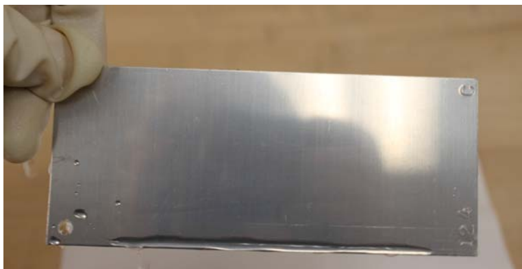
FIG. 2 Clean aluminum panel showing no water break. Water drains in a continuous sheet.
