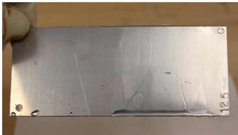
FIG. 4 Contaminated aluminum panel showing water-break on withdrawal from immersion. The water may break in a different pattern after each immersion of the same part.
