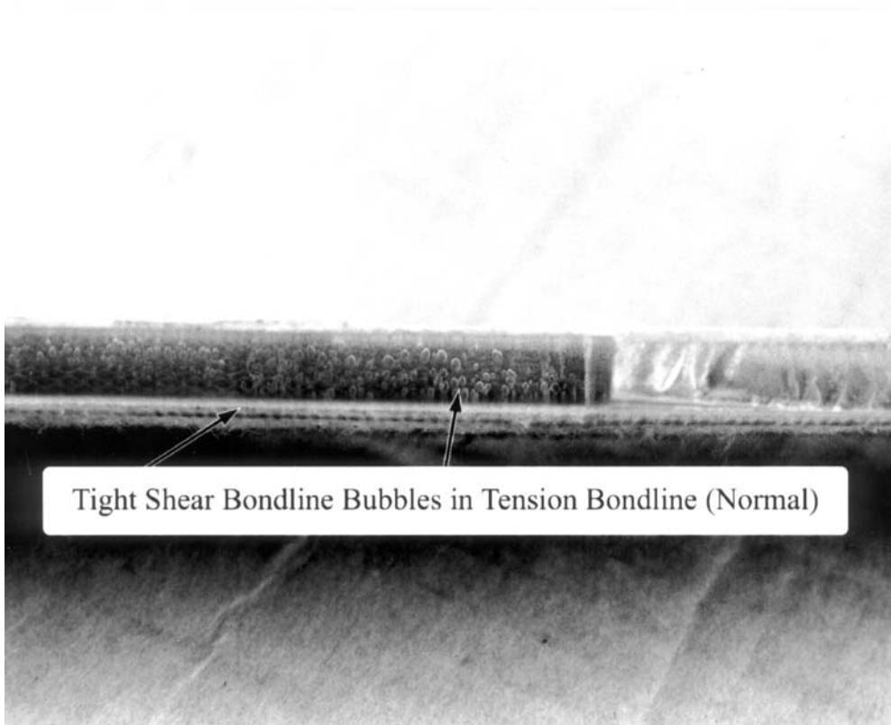
FIG. 3 Acceptable Air Bubbles (from Resin Curing)
