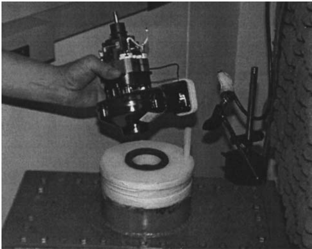
FIG. 2 Example of Standoff Pipe
