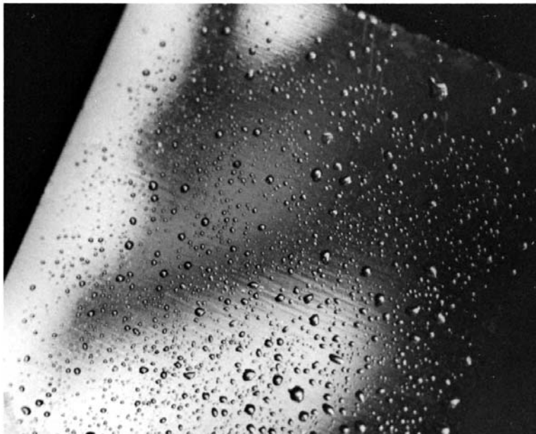
FIG. 6 Atomizer Test of Nickel Specimen with Hydrophobic Film Covering Surface (x2, Reduced One-Half in Reproduction)
