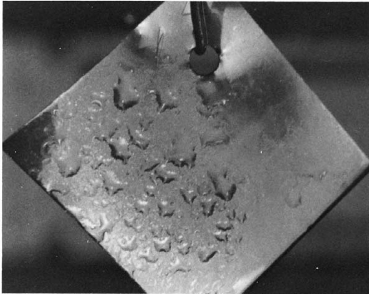
FIG. 5 Atomizer Test of Partially Contaminated Nickel specimen (x2, Reduced One-Half in Reproduction)
