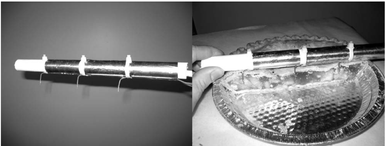
FIG. 2 Example Thermocouple Fixture for Measuring Pie Temperatures
