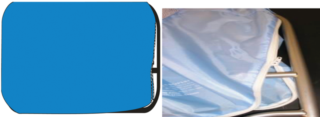
Bedrail fabric with a zipper that is not fully engaged. The zipper cannot be fully engaged due to interference with the middle bar.
