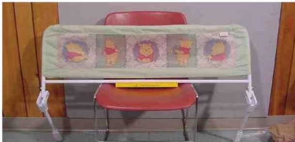
Bottom bar can be omitted from insertion into fabric sleeve or channel located at the base of the fabric component.
