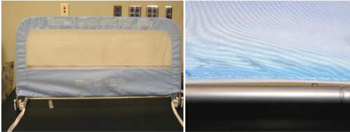
Bedrail fabric with bottom zipper misassembled, fabric cover can be zipped up without engaging the bottom horizontal bar.
