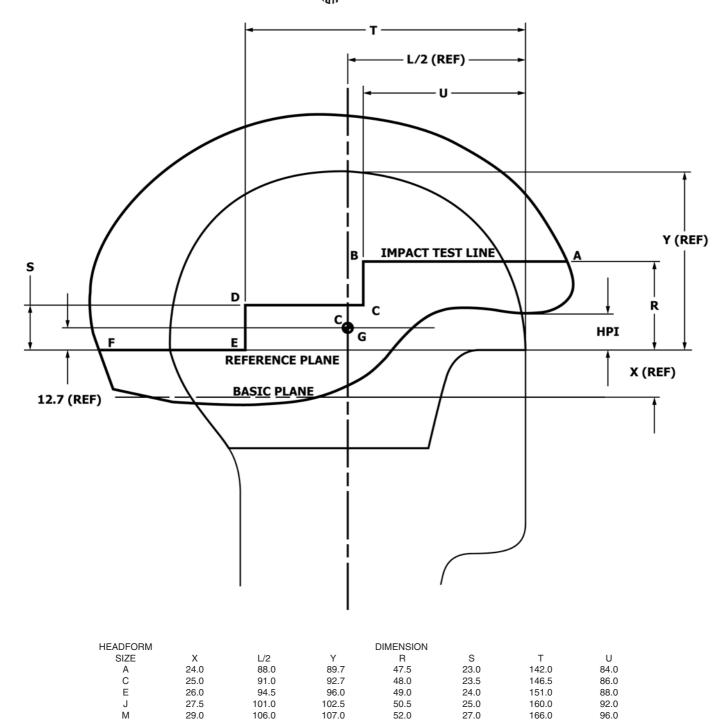
FIG. 1 Marking the Test Line
