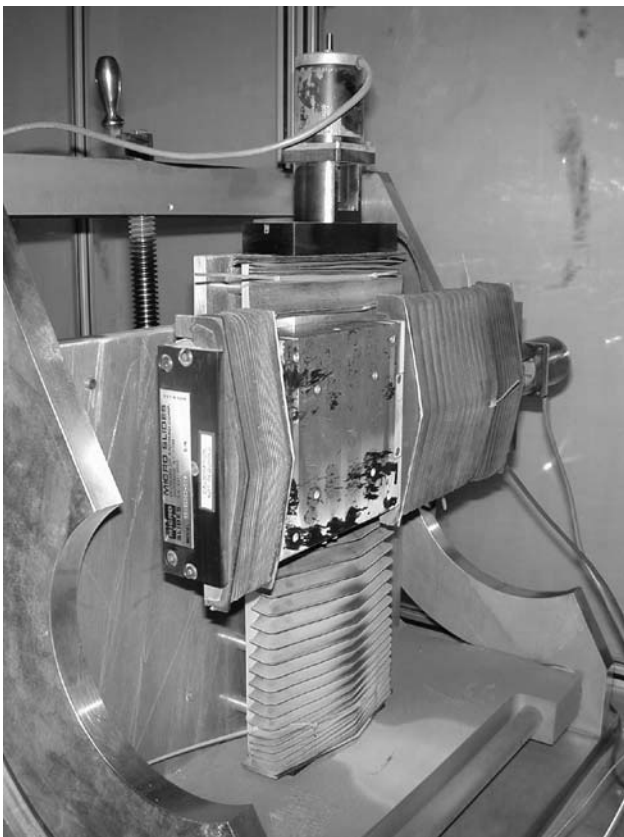
FIG. 7 Dust Erosion Test Bed with Programmable Stepper Motors
