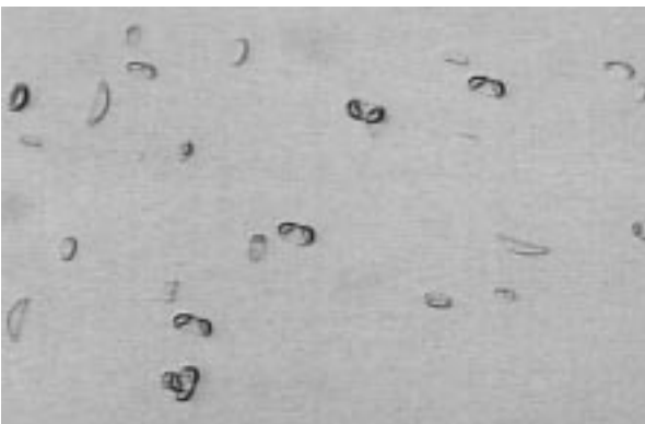
FIG. 11 Wright Etch With Agitation, Oxidation Stacking Fault, 500x, Low Resistivity Boron Doped, [100], (1100°C Steam, 80 minutes).
