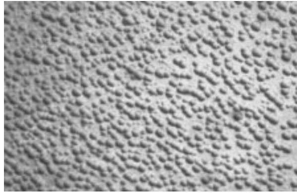
FIG. 18 Copper-3 Etch With Agitation, Shallow Pits (Haze), 500x, p type, 10 ohm-cm, [111], (1100°C Steam, 80 minutes), 2 \mu m removal
