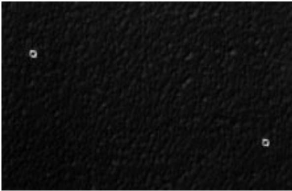
FIG. 4 Secco Etch With Agitation, Epitaxial Stacking Fault, 150x, [100], ~4 \mu\text{m} removal.
