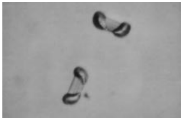
FIG. 20 Copper-3 Etch Without Agitation, Oxidation Stacking Fault, 1000x, p type, 10 ohm-cm, [100], (1100°C Steam, 80 minutes), 1 \mu m removal.
