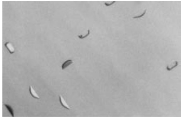
FIG. 8 Wright Etch With Agitation, Bulk Oxidation Stacking Fault, 500x, [100], (1100°C Steam, 80 minutes).
