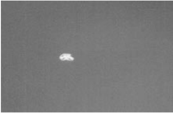
FIG. 5 Secco Etch With Agitation, Bulk Oxidation Stacking Fault, 200x, [100], (1100°C Steam, 80 minutes), ~15 \mu\text{m} removal.
