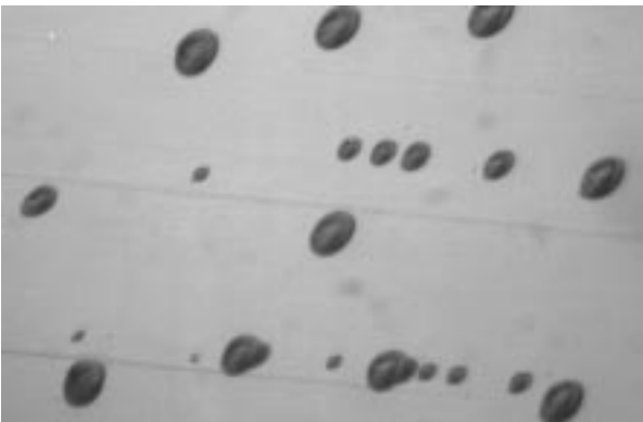
FIG. 22 Copper-3 Etch Without Agitation, Dislocations, 500x, p type, 10 ohm-cm, [100], 10 μm removal.
