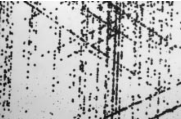
FIG. 23 Copper-3 Etch Without Agitation, Slip Dislocations, 100x, p type, 10 ohm-cm, [111], 10 μm removal.
