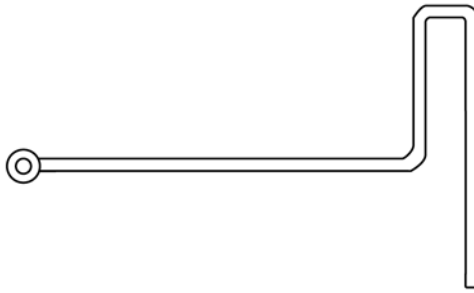
FIG. X2.1 Recommended EHPD Securing Clip
