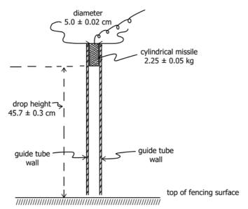
Note 1—Vertical projection of a schematic representation of the drop test is the basis of this performance specification. Whether a simple floor or a layer or strip placed over a floor, the distance from the starting position of the bottom of the missile to the top of the layer or strip, on which the fencing exercise is to occur, should measure 45.7  $\pm$  0.3 cm. The missile is guided by a vertical cylindrical guide tube.
