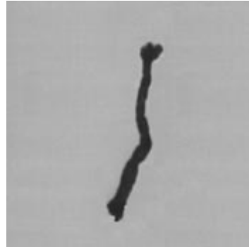
FIG. 57 Localized Lazer Scatterers, (Particle Contamination) in the Form of Small Fiber, Magnification 200 \times .
