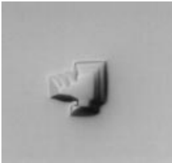
FIG. 62 Pit (Usually Associated With Insufficient Polishing of Caustic Etched Wafer), Magnification 1000×.
