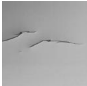
FIG. 47 Relatively Small Edge Chips on a Polished Edge Face, Magnification 200 \times .
