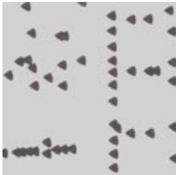
FIG. 1 Dislocation Etch Pits on (111) Silicon, Following 3-Min Sirtl Etch, Magnification 110×.
