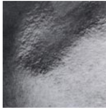
FIG. 64 Saw Blade Defect Seen on Lapped and Etched Wafer, Magnification 6×.
