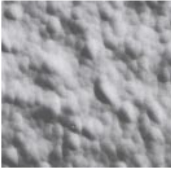
FIG. 60 Orange Peel Surface Roughness, Magnification 200×.
