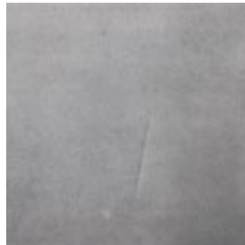
FIG. 53 Groove or Micro-Scratch, Magnification 220 \times .
