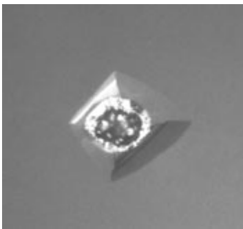
FIG. 50 Epitaxial Large Point Defect, No Preparation Required, Magnification 200 \times .
