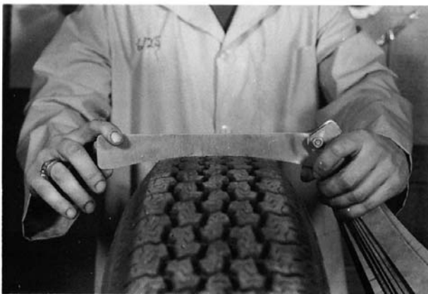
FIG. 5 Tread Radius Measurement
