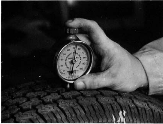
FIG. 9 Tread Hardness Measurement
