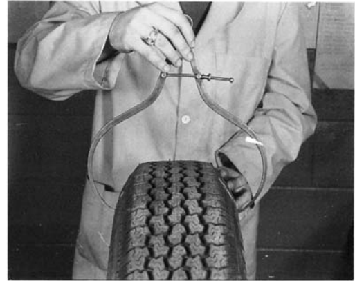
FIG. 3 Overall Width Measurement
