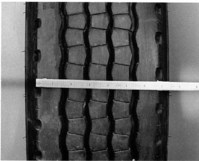
FIG. 10 Tread Arc Width Measurement
