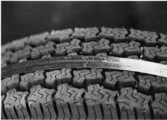
FIG. 2 Outside Diameter Measurement
