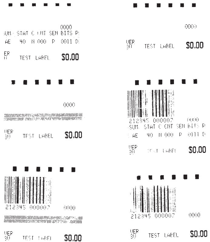
FIG. 3 Hobart 18VP Thermal Printer, 2 Diagnostic Test Pattern
