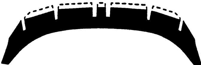
FIG. 2 Uniform or Regular Wear
