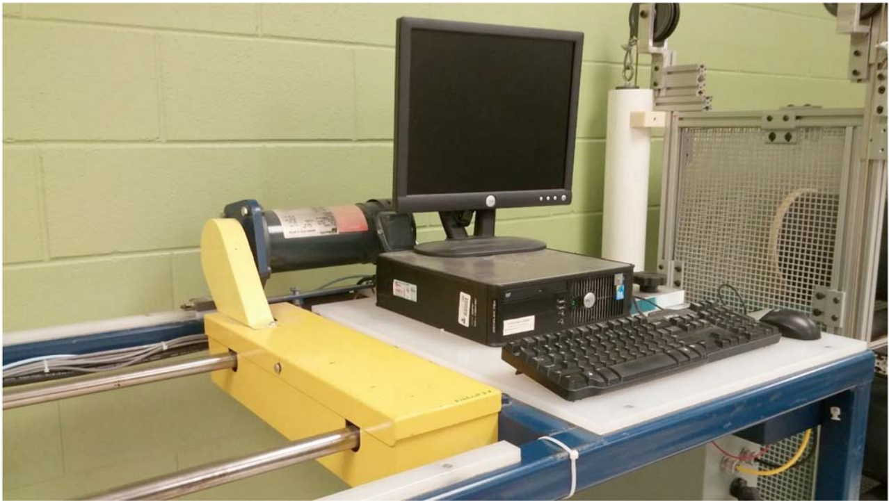
FIG. 3 Motion Drive and Data Collection Computer
