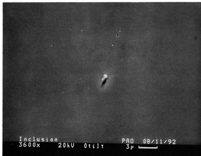
FIG. 2 Example of Pit Defect (3600 × magnification)
