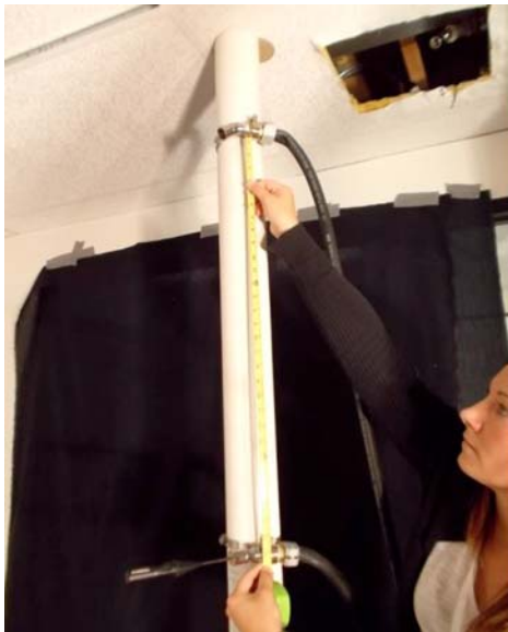
FIG. A1.9 Locating Height of Top Spray Nozzle with Respect to Middle Spray Nozzle
