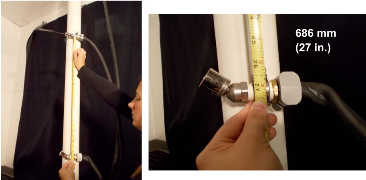
FIG. A1.10 Locating Height of Bottom Spray Nozzle with Respect to Middle Spray Nozzle
