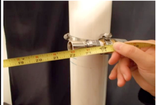
FIG. A1.5 Measuring Distance from Central Nozzle to Center Manikin Target
