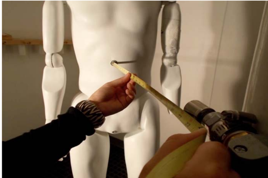
FIG. A1.6 Measuring Distance from Central Nozzle to Center Manikin Target—View 2
