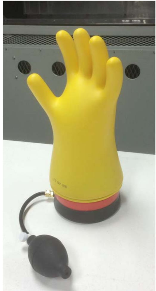
FIG. 51 Inflator – 11 in. Glove Length
