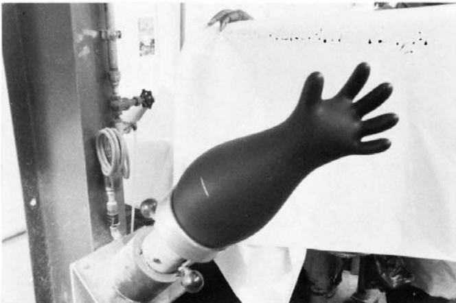
FIG. 50 Inflator (Glove Inflated to Maximum Allowable Degree)
