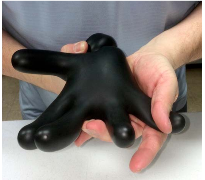
FIG. 38 Inspection – Between Fingers/Twirled Glove
