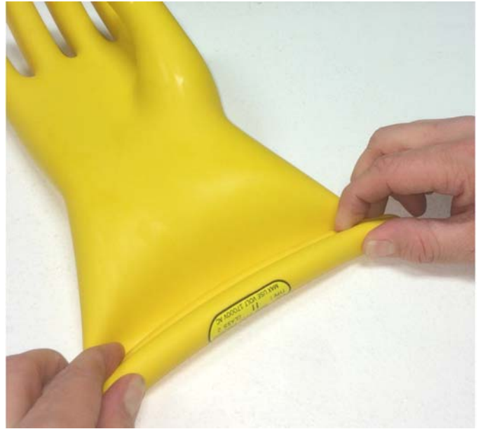
FIG. 46 Rolling – Sealing the Edges
