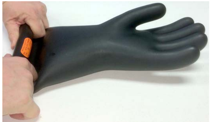
FIG. 47 Rolling – Trapping the Air
