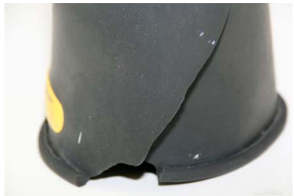
FIG. 29 Tear Rubber Glove
