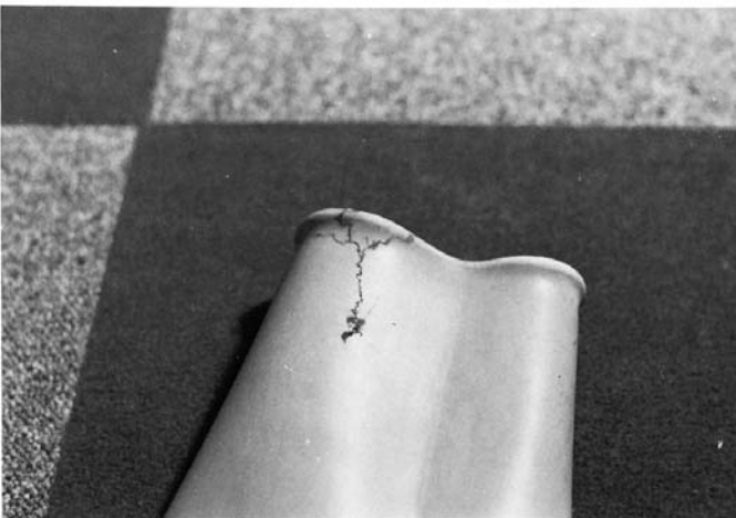
FIG. 32 Tracking—Insufficient Immersion Depth
