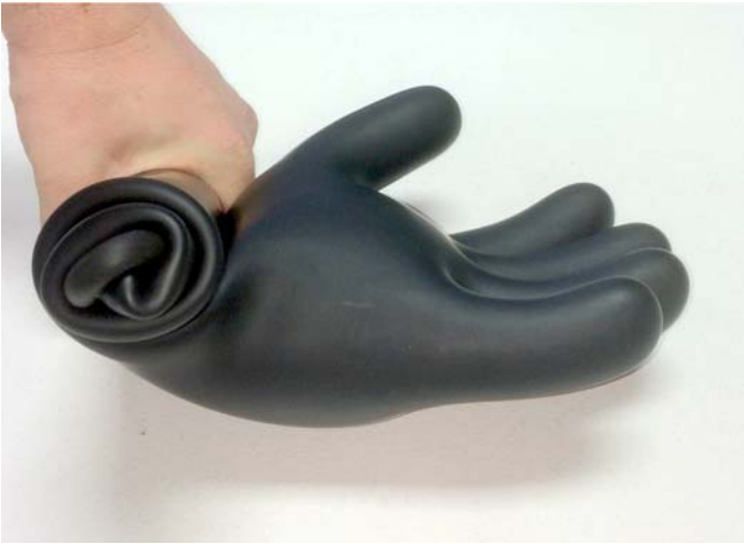
FIG. 49 Inspection – 14 in. Glove Length
