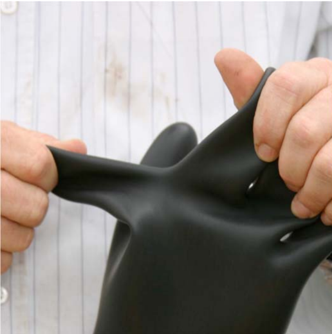
FIG. 37 Inspection – Between Fingers
