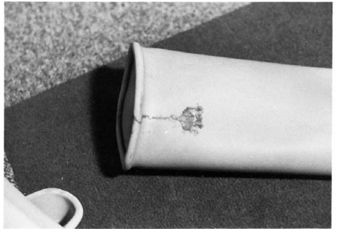
FIG. 33 Tracking—Contaminated Dielectric Fluid
