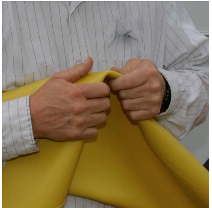
FIG. 34 Inspection – Sleeve Pinch Rolling
