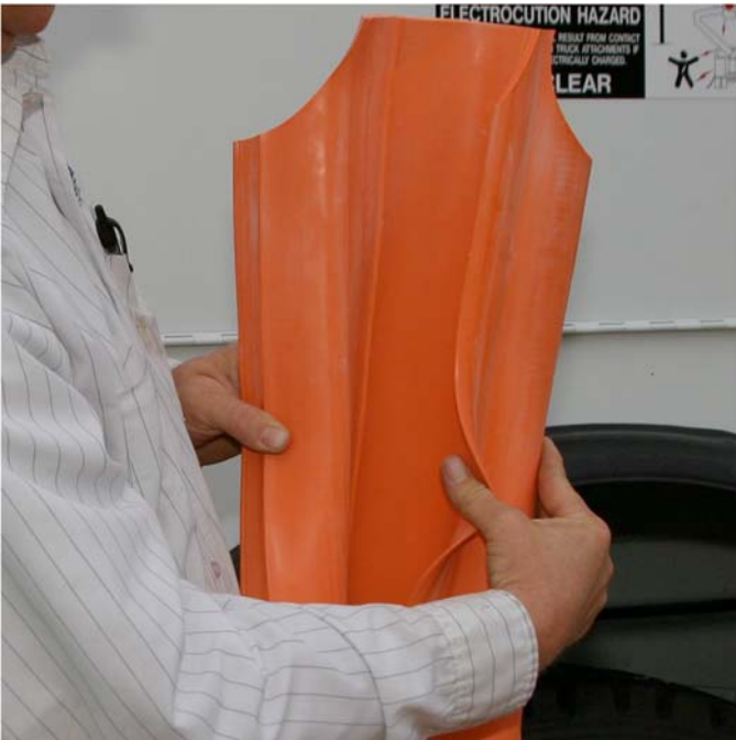
FIG. 40 Inspection – Inside Line Hose
