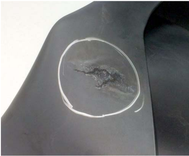
FIG. 31 Tracking—Burned Rubber Sleeve
