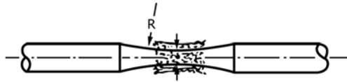
FIG. 6 Specimens With a Continuous Radius Between the Ends for Rotating Beam or Axial loading
